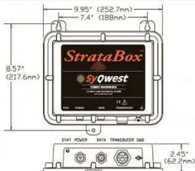
The diagram shows the physical dimensions of the StrataBox unit. It is a rectangular device with a handle on top. The front panel has a display screen and several control buttons. Dimensions are labeled as follows: Height: 8.57" (217.6mm), Width: 9.95" (252.7mm), Depth: 7.4" (188mm), and a side dimension of 2.45" (62.2mm).
